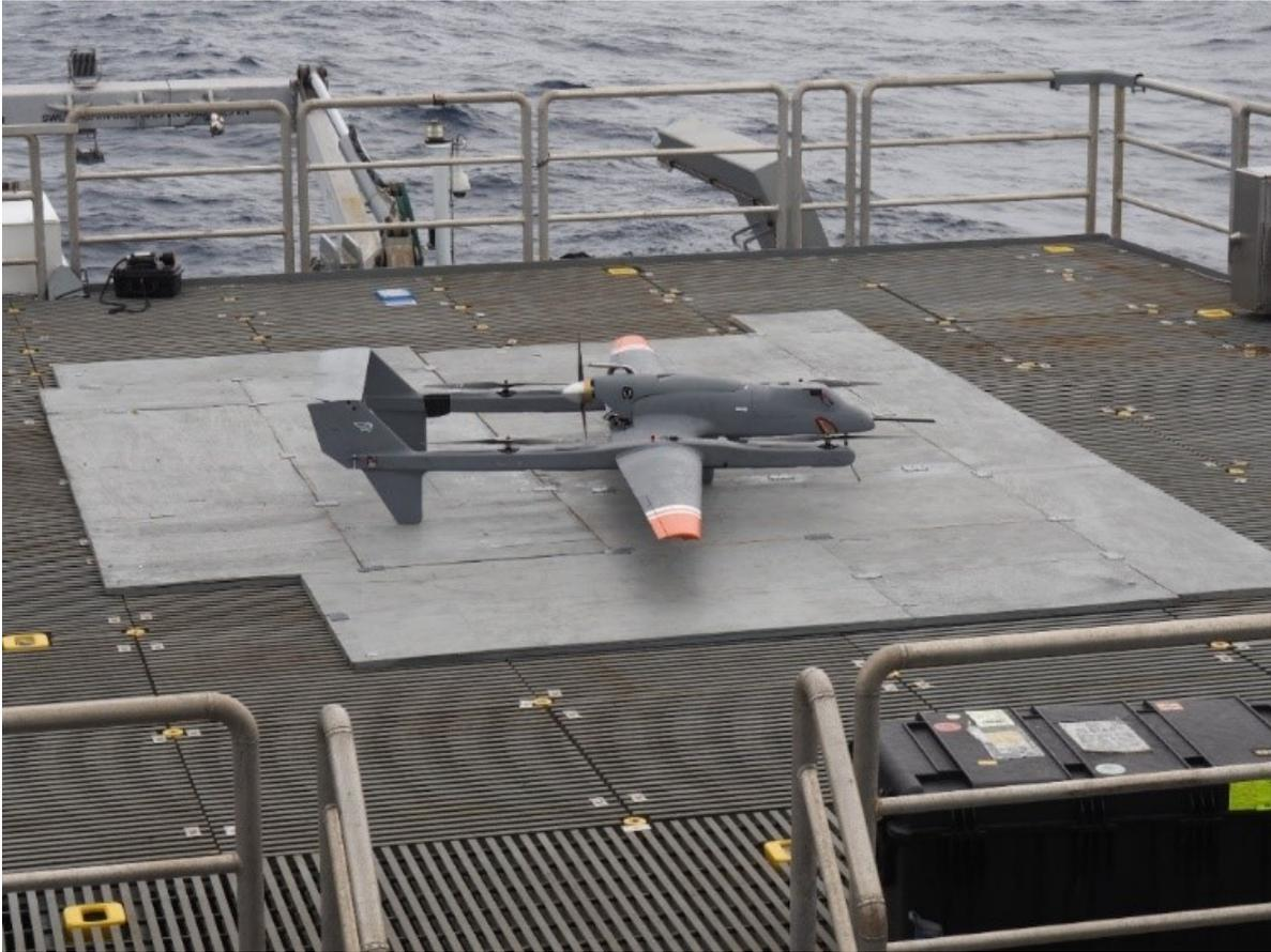
*Figure 3. Latitude Engineering Hybrid Quadrotor model HQ-90 with vertical takeoff and landing (VTOL) capability.*
