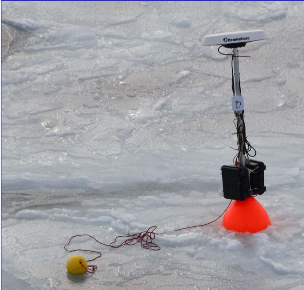
*Figure 2. Stand-Alone USBL Positioning Buoy, here seen in newly formed frazil ice in the Barents Sea 2017.*
