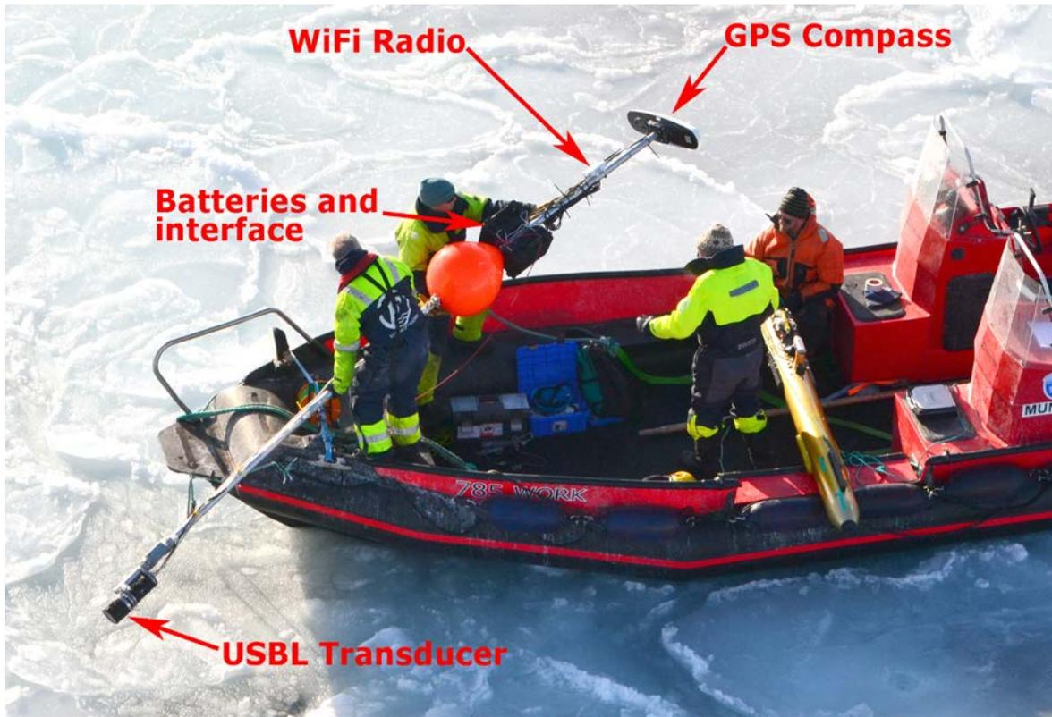
*Figure 1. Stand-Alone USBL Positioning Buoy and Gavia AUV in boat.*
